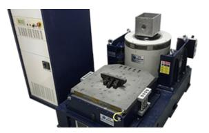
Incorporating a climatic chamber, vibration table, and altitude test chamber, we are able to test our products to exacting standards for shock, vibration, temperature and humidity. In addition, we can simulate the low pressure conditions of >50,000ft as required for some of our antenna units.
